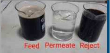
Figure 3. Feed, Permeate, and reject samples when treating Textile wastewater with FilmTec™ Fortilife™ XC120.
