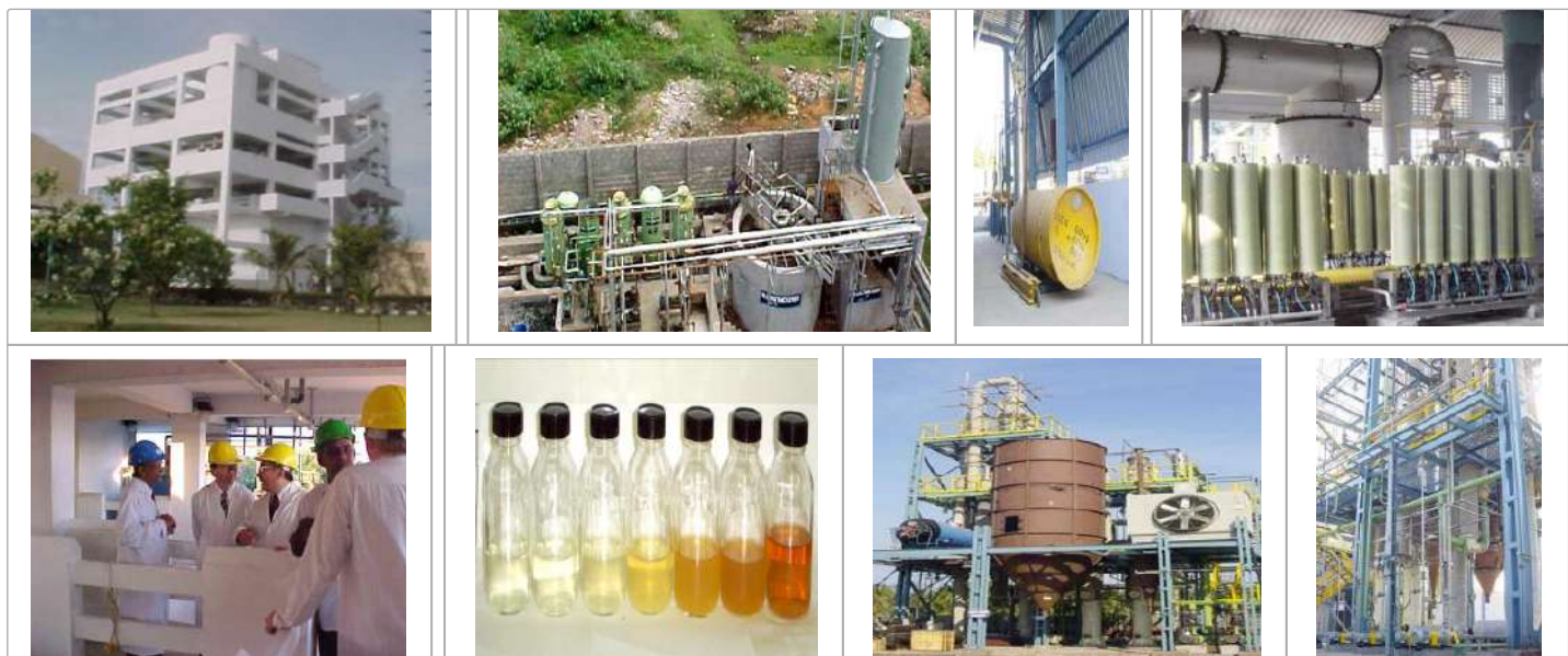
Fig.2. Clockwise from top left. The multi-tier ETP with stripper tower at top, tertiary filtration, oxidation by chlorination, desalination by disc & tube membranes, thermal evaporator, crystallizer, colour removal in the sequence, the lead author with buyers's inspectors from overseas.
