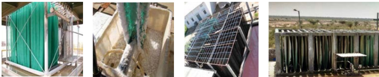
Fig.4. Left and second The Israeli WAIV evaporator with simple drop sheets and which can crystallize the salt by controlled evaporation. Third and fourth. Two such installations in India not conceded by the respective PCBs and favored to provide mechanical thermal evaporators
