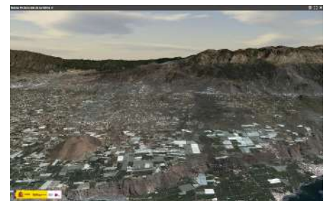
Image 2: CNIG used ContextCapture to integrate 14,000 drone-captured images with low-resolution photographs into a single, accurate digital twin. Image courtesy of Spanish National Center for Geographic Information. The digital twin enabled CNIG to virtually study the area, plan new infrastructure development, and define protection and management plans to safeguard people in the area from future eruptions.
