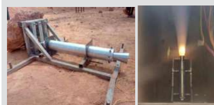
Image 4: Rocket thrust assessment with thrustMIT via solid motor test.
