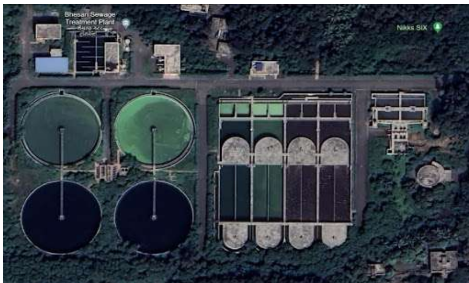
Fig.1-Ovivo's advanced Oxidation Ditch Google earth Image
