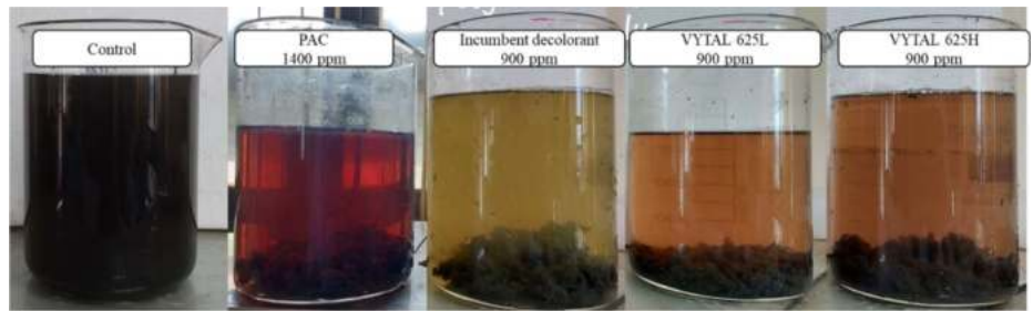
Fig. 1 Treated effluent photo at optimized dosage
