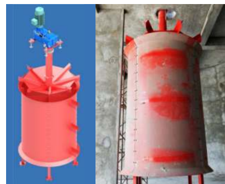
Fig.3-LSC Aerator w/Draft Tube
